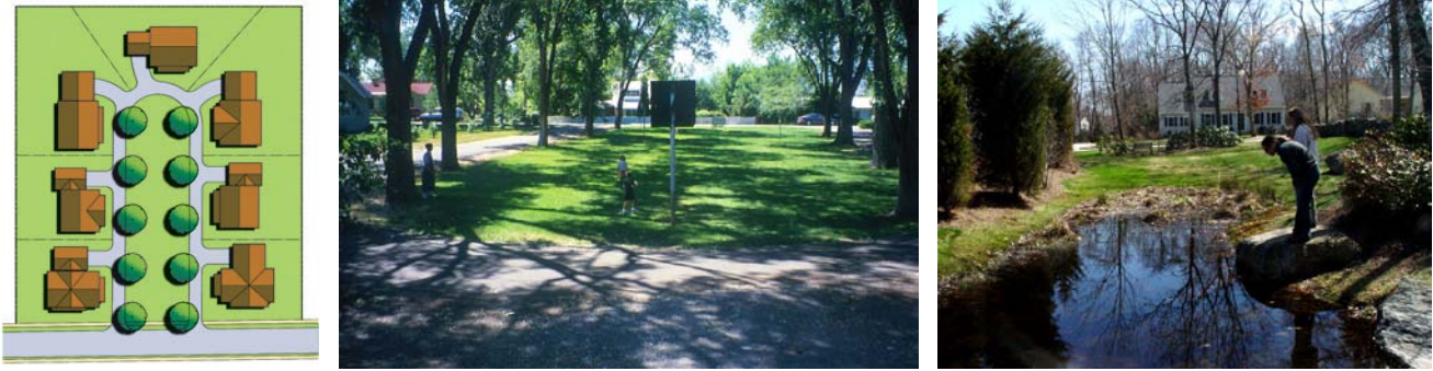
Figures 14, 15, and 16 The “court” or “close”, pictured in the above sketch, is essentially a short cul-de-sac with a central boulevard median, greatly expanded in width to serve various functions, from aesthetic enhancement to stormwater management. The central open space is bounded by a one-way circulatory street, and provides a green oasis with much scope for shade tree planting and stormwater management – plus a safe place for young residents to recreate informally.
