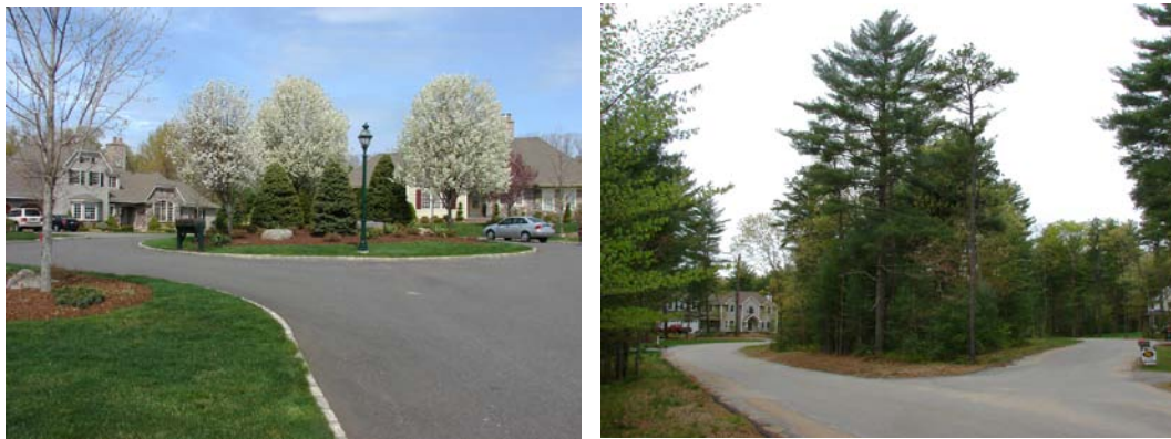
Figures 17 and 18 When the above concept is not feasible, cul-de-sacs should at least be terminated with an island planted with canopy shade trees to properly fill the “celestial space” above this wide bulbous street form. Or existing trees can be left in place. Plowing snow is much easier because plow operators can make one efficient sweep around the central island.
